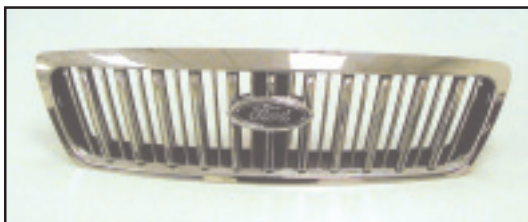
Chromate treatment parts alternative plan -chromate treatment material replacement to reduce use of substances of concern
